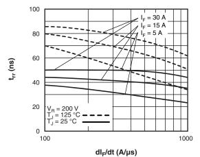
Fig. 5 - Typical Reverse Recovery Time vs. dl<sub>F</sub>/dt
