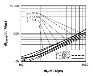
Fig. 8 - Typical dl<sub>(rec)M</sub>/dt vs. dl<sub>F</sub>/dt
