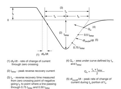
Fig. 10 - Reverse Recovery Waveform and Definitions
