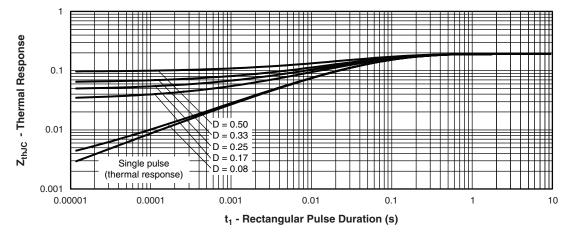
Fig. 9 - Maximum Thermal Impedance  $Z_{\text{thJC}}$  Characteristics
