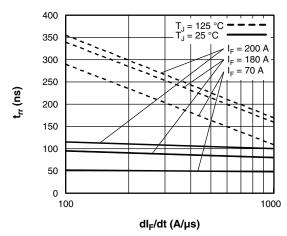
Fig. 5 - Typical Reverse Recovery Time vs. dl<sub>F</sub>/dt
