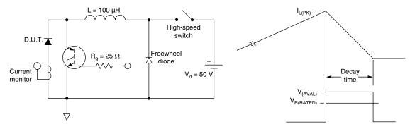
Fig. 12 - Avalanche Test Circuit and Waveforms
