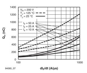
Fig. 7 - Typical Stored Charge vs. dl<sub>F</sub>/dt
