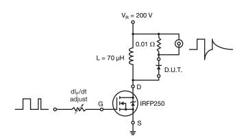
Fig. 9 - Reverse Recovery Parameter Test Circuit
