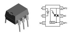
The IL4116/ IL4117/ IL4118 uses zero cross line voltage detection circuit witch consists of two enhancement MOSFETS and a photodiode. The inhibit voltage of the network is determined by the enhancement voltage of the N-channel FET. The P-channel FET is enabled by a photocurrent source that permits the FET to conduct the main voltage to gate on the Nchannel FET. Once the main voltage can enable the N-channel, it clamps the base of the phototransistor, disabling the first stage SCR predriver.
