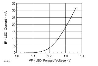
Figure 1. LED Forward Current vs.Forward Voltage
