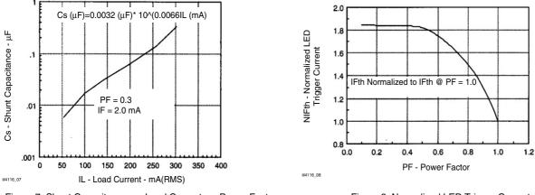
Figure 7. Shunt Capacitance vs. Load Current vs. Power Factor
