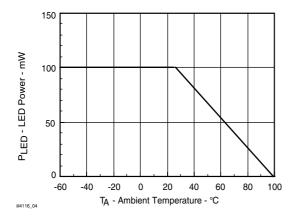
Figure 4. Maximum LED Power Dissipation
