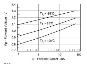
Figure 2. Forward Voltage vs. Forward Current
