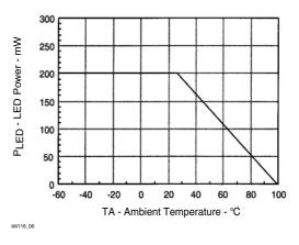
Figure 6. Maximum Output Power Dissipation
