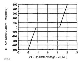
Figure 5. On-State Terminal Voltage vs. Terminal Current
