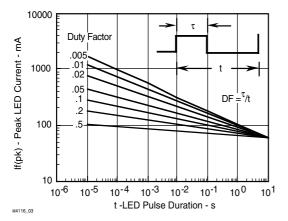
Figure 3. Peak LED Current vs. Duty Factor, Tau
