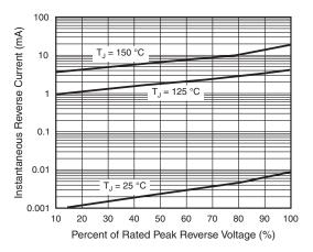
Fig. 4 - Typical Reverse Characteristics
