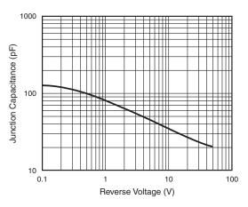
Fig. 5 - Typical Junction Capacitance
