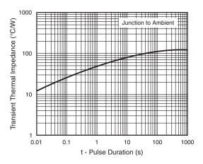
Fig. 6 - Typical Transient Thermal Impedance
