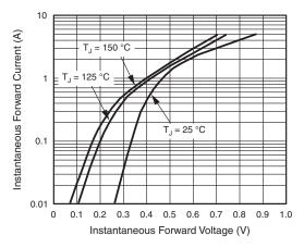
Fig. 3 - Typical Instantaneous Forward Characteristics
