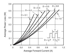
Fig. 2 - Forward Power Loss Characteristics
