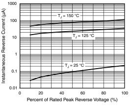
Fig. 4 - Typical Reverse Characteristics
