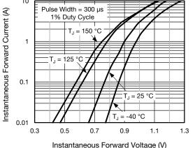
Fig. 3 - Typical Instantaneous Forward Characteristics
