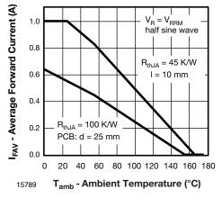
Fig. 2 - Max. Average Forward Current vs. Ambient Temperature
