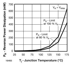
Fig. 4 - Max. Reverse Power Dissipation vs. Junction Temperature
