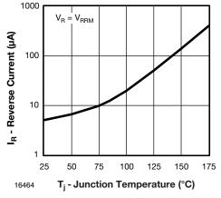
Fig. 3 - Reverse Current vs. Junction Temperature
