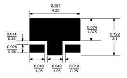
FIGURE 1. Recommended Copper Spreading Footprint
