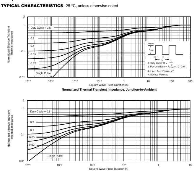
Normalized Thermal Transient Impedance, Junction-to-Foot
