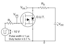
Fig. 10a - Switching Time Test Circuit
