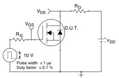
Fig. 10a - Switching Time Test Circuit
