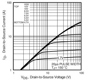
Fig. 2 - Typical Output Characteristics
