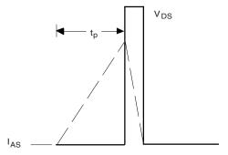
Fig. 12b - Unclamped Inductive Waveforms
