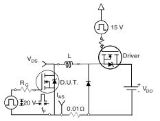
Fig. 12a - Unclamped Inductive Test Circuit
