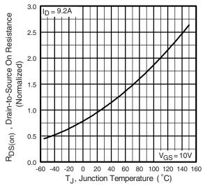
Fig. 4 - Normalized On-Resistance vs. Temperature
