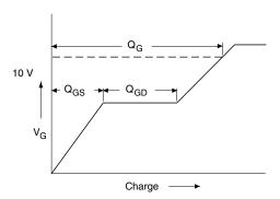
Fig. 13a - Basic Gate Charge Waveform
