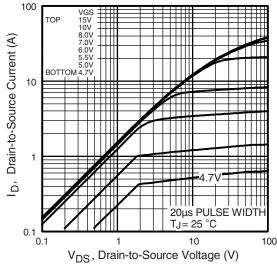
Fig. 1 - Typical Output Characteristics
