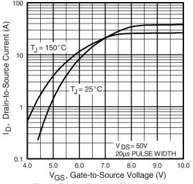
Fig. 3 - Typical Transfer Characteristics
