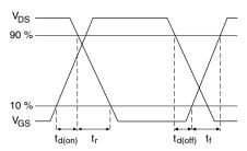
Fig. 10b - Switching Time Waveforms
