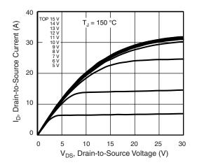
Fig. 2 - Typical Output Characteristics
