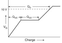
Fig. 17 - Basic Gate Charge Waveform
