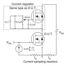
Fig. 18 - Gate Charge Test Circuit
