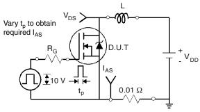
Fig. 15 - Unclamped Inductive Test Circuit
