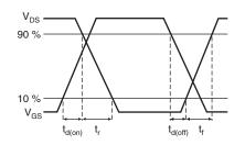
Fig. 14 - Switching Time Waveforms
