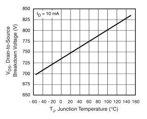
Fig. 11 - Temperature vs. Drain-to-Source Voltage
