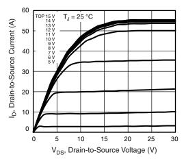
Fig. 1 - Typical Output Characteristics
