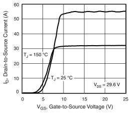
Fig. 3 - Typical Transfer Characteristics
