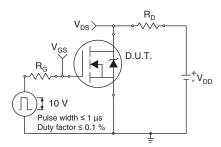
Fig. 13 - Switching Time Test Circuit
