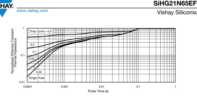
Fig. 12 - Normalized Thermal Transient Impedance, Junction-to-Case
