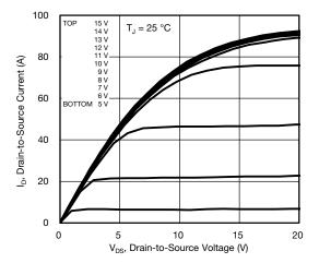
Fig. 1 - Typical Output Characteristics
