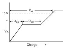
Fig. 17 - Basic Gate Charge Waveform
