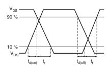
Fig. 14 - Switching Time Waveforms
