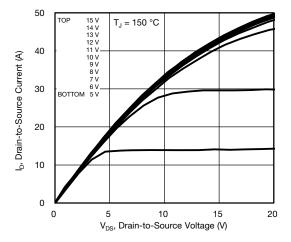
Fig. 2 - Typical Output Characteristics
