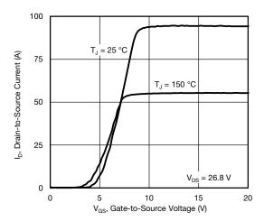
Fig. 3 - Typical Transfer Characteristics
