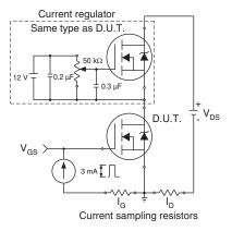
Fig. 18 - Gate Charge Test Circuit
