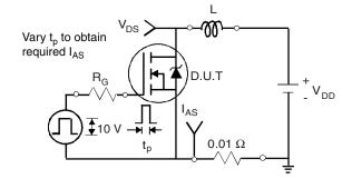
Fig. 15 - Unclamped Inductive Test Circuit
