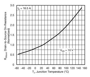
Fig. 4 - Normalized On-Resistance vs. Temperature
