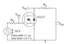
Fig. 10a - Switching Time Test Circuit
