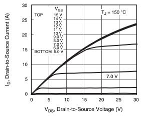
Fig. 2 - Typical Output Characteristics (TO-220)
