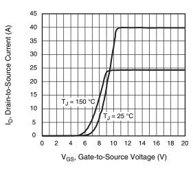
Fig. 3 - Typical Transfer Characteristics
