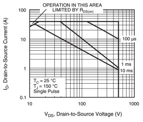
Fig. 8 - Maximum Safe Operating Area (TO-220AB, D2PAK)
