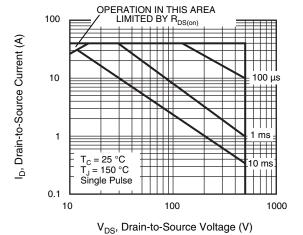
Fig. 9 - Maximum Safe Operating Area (TO-220 FULLPAK)
