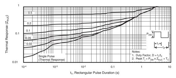
Fig. 12 - Maximum Effective Transient Thermal Impedance, Junction-to-Case (TO-220 FULLPAK)
