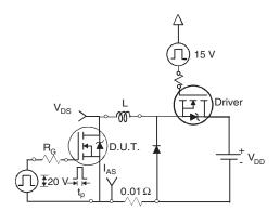
Fig. 13a - Unclamped Inductive Test Circuit
