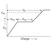
Fig. 14a - Basic Gate Charge Waveform
