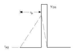
Fig. 13b - Unclamped Inductive Waveforms
