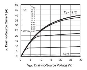
Fig. 1 - Typical Output Characteristics (TO-220)
