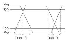
Fig. 10b - Switching Time Waveforms
