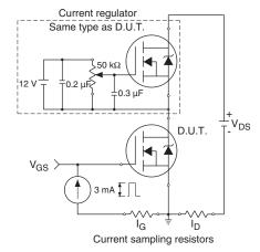
Fig. 14b - Gate Charge Test Circuit
