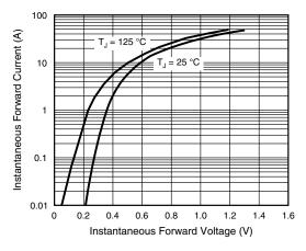
Fig. 3 - Typical Instantaneous Forward Characteristics
