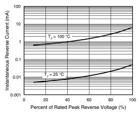
Fig. 4 - Typical Reverse Current Characteristics
