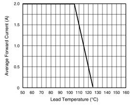
Fig. 1 - Forward Derating Curve
