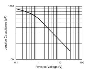
Fig. 5 - Typical Junction Capacitance
