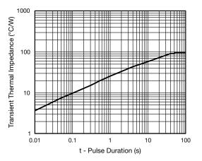
Fig. 6 - Typical Transient Thermal Impedance
