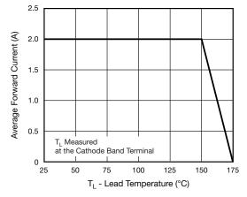
Fig. 1 - Forward Current Derating Curve
