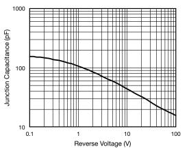
Fig. 5 - Typical Junction Capacitance
