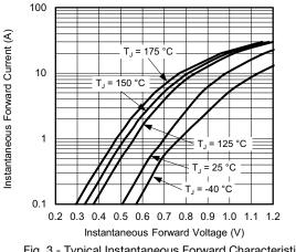
Fig. 3 - Typical Instantaneous Forward Characteristics
