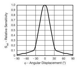
Fig. 6 - Relative Radiant Intensity vs. Angular Displacement
