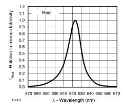
Figure 2. Relative Intensity vs. Wavelength
