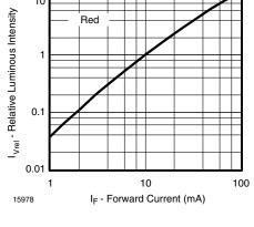
Figure 5. Relative Luminous Flux vs. Forward Current
