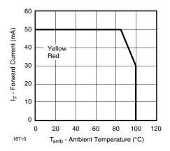
Figure 1. Forward Current vs. Ambient Temperature
