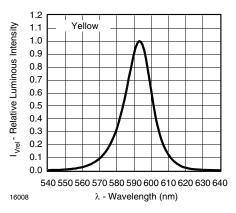
Figure 3. Relative Intensity vs. Wavelength
