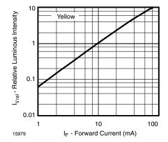
Figure 6. Relative Luminous Flux vs. Forward Current
