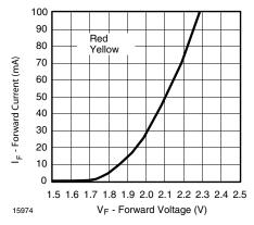
Figure 4. Forward Current vs. Forward Voltage
