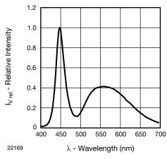
Fig. 3 - Relative Intensity vs. Wavelength
