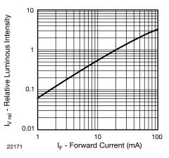
Fig. 5 - Relative Luminous Intensity vs. Forward Current
