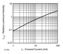
Figure 5. Relative Luminous Flux vs. Forward Current
