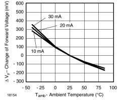
Figure 7. Change of Forward Voltage vs. Ambient Temperature
