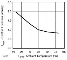
Figure 6. Relative Luminous Intensity vs. Amb. Temperature
