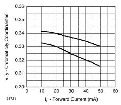
Figure 9. Chromaticity Coordinate Shift vs. Forward Current
