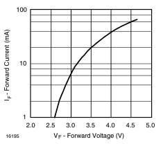
Figure 4. Forward Current vs. Forward Voltage
