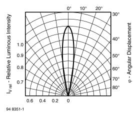
Figure 2. Relative Luminous Intensity vs. Angular Displacement
