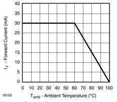
Figure 1. Forward Current vs. Ambient Temperature
