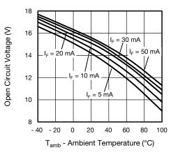
Fig. 5 - Open Circuit Voltage vs. Ambient Temperature
