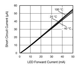
Fig. 3 - Short Circuit Current vs. LED Forward Current
