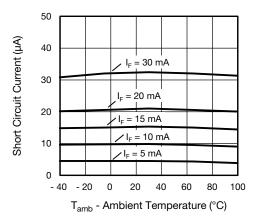
Fig. 4 - Short Circuit Current vs. Ambient Temperature
