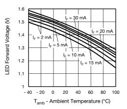
Fig. 6 - LED Forward Voltage vs. Ambient Temperature
