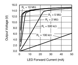
Fig. 2 - Output Voltage vs-LED Current
