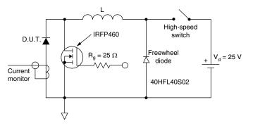
Fig. 8 - Unclamped Inductive Test Circuit
