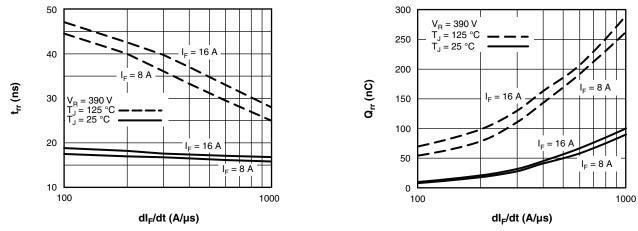
Fig. 7 - Typical Reverse Recovery Time vs. dI<sub>F</sub>/dt
