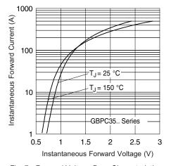
Fig. 7 - Forward Voltage Drop Characteristics
