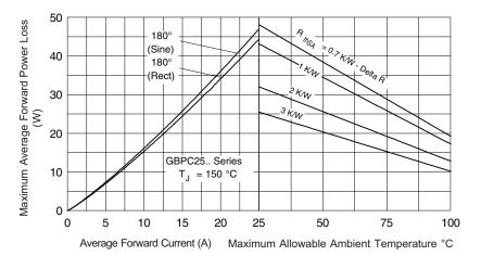
Fig. 3 - Total Power Loss Characteristics
