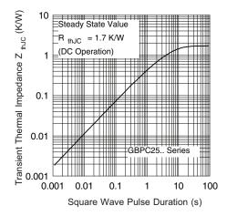
Fig. 11 - Thermal Impedance Z<sub>thJC</sub> Characteristic
