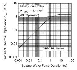
Fig. 12 - Thermal Impedance Z<sub>thJC</sub> Characteristic
