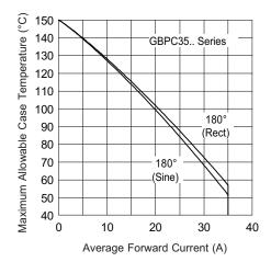
Fig. 6 - Current Ratings Characteristics
