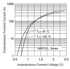
Fig. 2 - Forward Voltage Drop Characteristics
