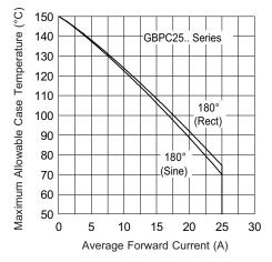
Fig. 1 - Current Ratings Characteristics
