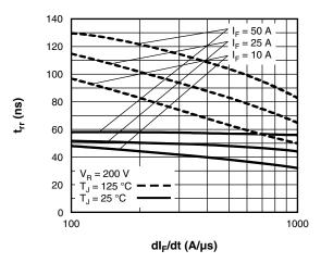
Fig. 5 - Typical Reverse Recovery Time vs. dl<sub>E</sub>/dt
