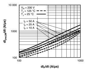
Fig. 8 - Typical dl<sub>(rec)M</sub>/dt vs. dl<sub>F</sub>/dt
