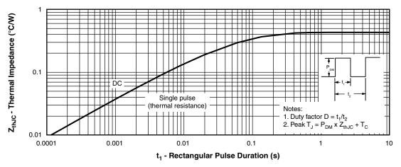
Fig. 4 - Maximum Thermal Impedance Z<sub>thJC</sub> Characteristics (Per Diode)
