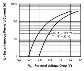
Fig. 1 - Typical Forward Voltage Drop Characteristics (Per Diode)
