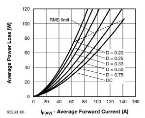
Fig. 6 - Forward Power Loss Characteristics
