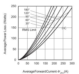
Fig. 6 - Forward Power Loss Characteristics
