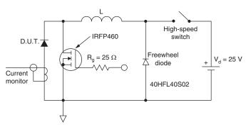
Fig. 8 - Unclamped Inductive Test Circuit
