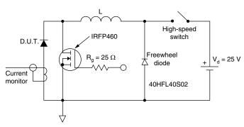
Fig. 8 - Unclamped Inductive Test Circuit
