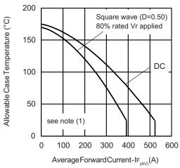
Fig. 5 - Maximum Allowable Case Temperature vs.
