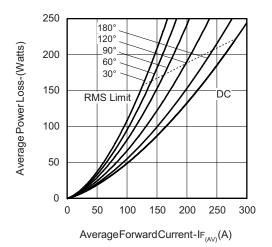
Fig. 6 - Forward Power Loss Characteristics
