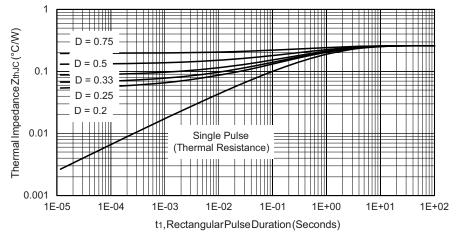
Fig. 4 - Maximum Thermal Impedance Z<sub>thJC</sub> Characteristics
