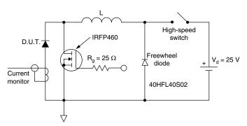
Fig. 8 - Unclamped Inductive Test Circuit
