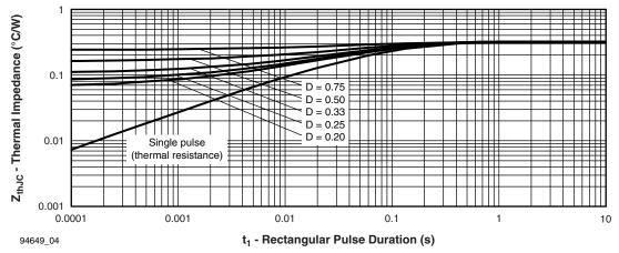
Fig. 4 - Maximum Thermal Impedance Z<sub>thJC</sub> Characteristics (Per Diode)
