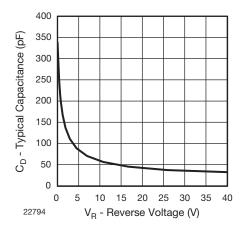
Fig. 3 - Typical Capacitance vs. Reverse Voltage
