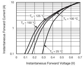
Fig. 3 - Typical Instantaneous Forward Characteristics
