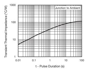
Fig. 6 - Typical Transient Thermal Impedance
