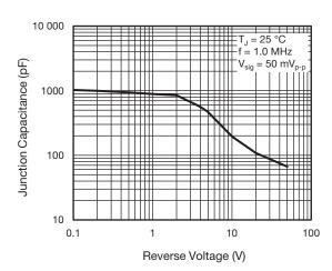
Fig. 5 - Typical Junction Capacitance
