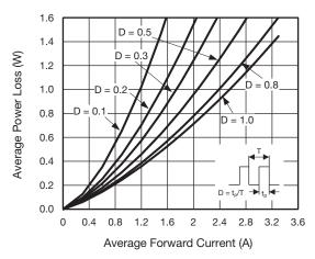
Fig. 2 - Forward Power Loss Characteristics
