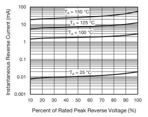
Fig. 4 - Typical Reverse Leakage Characteristics
