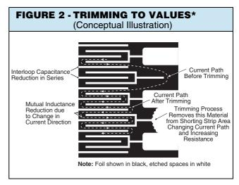
\* To acquire a precision resistance value, the Bulk Metal® Foil chip is trimmed by selectively removing built-in "shorting bars." To increase the resistance in known increments, marked areas are cut, producing progressively smaller increases in resistance. This method eliminates "hot spot" and improves the long term stability of the resistor.
