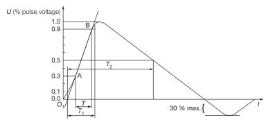
$\begin{array}{ll} \mbox{Front time:} & T_1 = 1.67 \ x \ T = 1.2 \ \mu s \pm 30 \ \% \\ \mbox{Time to half-value:} & T_2 = 50 \ \mu s \pm 20 \ \% \end{array}$
