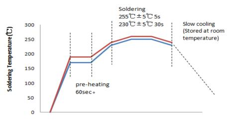
Reflow soldering method:
