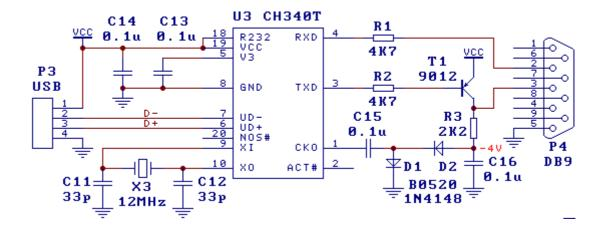
The figure above also shows that USB is converted to RS232. This circuit has the same function as the circuit shown in Section 7.2 except the range of output RS232 is narrower. When R232 pin is driven high, the assistant RS232 function will be enabled, just need to add some diodes, transistors, resistors and capacitors, the special level converter chip U5 in Section 7.2 could be replaced and the hardware cost is lower.
