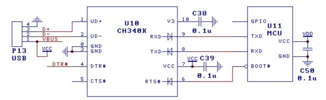
The figure above shows the reference circuit of MCU connecting to CH340K through TTL UART to realize USB communication under dual power supply mode. The CH340K is powered by the USB bus, VBUS (VCC), and the MCU uses another power supply VDD, which supports 5V, 3.3V or even 2.5V and 1.8V. The EPAD of CH340K is an optional GND pin, which can be easily connected to GND or not connected according to PCB routing.
