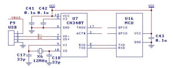
The figure above is a reference design to achieve USB connection on an MCU by connecting it to a CH340 via TTL UART. Here self-power mode is selected, VCC supports 5V or 3.3V (V3 shorted to VCC if VCC is 3.3V), and USB bus power (VBUS) is not used at all (Can be tested by connecting series resistor to I/O of MCU if needed). CH340 shares the same power source with MCU, hence there would be no current inrush
