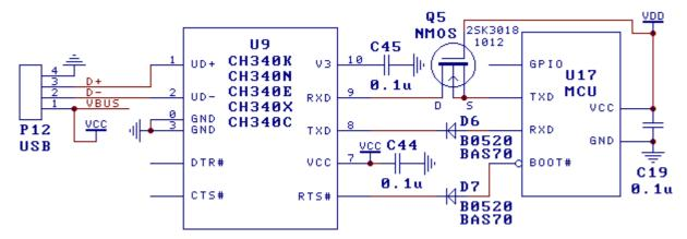
The figure above is a reference design to achieve USB connection on an MCU by connecting it to a CH340 via TTL UART. CH340 is powered by USB bus VBUS. MCU is powered by another power source VDD, VDD supports 5V, 3.3V and even 2.5V, 1.8V.
