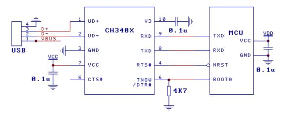
The figure above shows the reference circuit for one-click download based on a multi-mode USB to UART MCU, without manual setting or manual reset.
