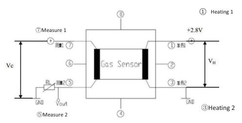
Fig2. GM-302B test circuit
