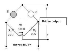
Fig2. Basic Test Circuit
