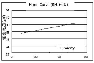
Fig8. Sensitivity at different humidity
