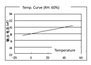
Fig6. Sensitivity at different temp.
