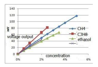
Fig3. Sensitivity Curve
