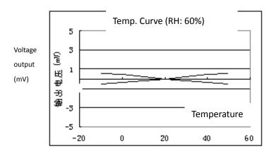
Fig5.Zero point at different temp.
