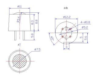
Fig1. Sensor Structure
