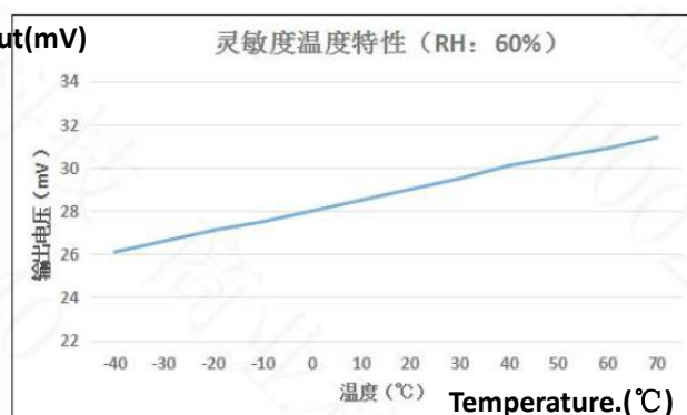
Fig6. Sensitivity at different temp.
