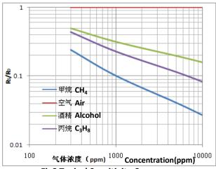
Fig3.Typical Sensitivity Curve
