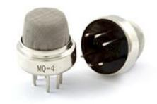
MQ-4 gas sensor has high sensitivity to methane, also has anti-interference to alcohol and other gases.
