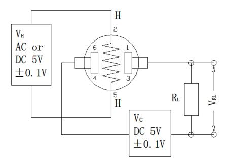
Fig2. MQ-4 Test Circuit
