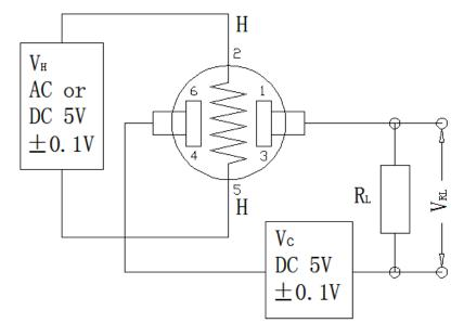
Fig2. MQ-8 Test Circuit
