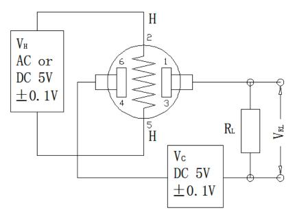
Fig2. MQ131 Test Circuit
