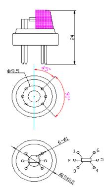
Fig1.Sensor Structure Unit: mm
