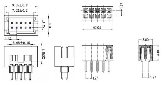
Fig2.Terminal Type (PH=2x5x1.27mm) Fig2-1Matching Terminal Description: for reference only **NOTE.** If users choose surfaced mount, please be sure about the safety distance between sensor's housing and terminal pins, avoiding short circuit or other malfunction.
