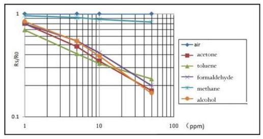
Contrast of the sensitivity in different gases
