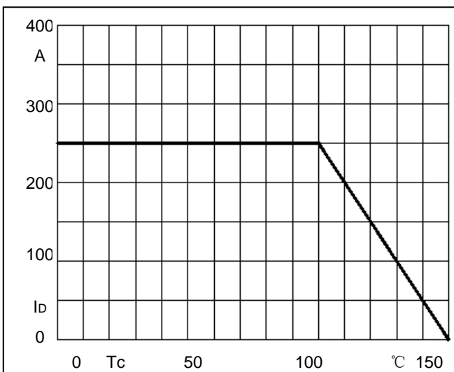
Fig5. Forward Current Derating Curve
